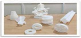
Components manufactured using FDM
